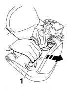
11.After the pulsating action has stopped in the brake lever, it is generated in the brake pedal "1" 0.5 second later and continues for approximately 2.5 seconds.
